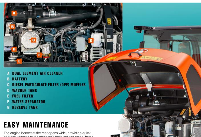
The engine bonnet at the rear opens wide, providing quick and easy access to the machine's main service areas. Items that require routine maintenance and service are within easy reach for fast and simple servicing. Quick-open panels on the right and left sides provide speedy access to the fuel refill (right side) and battery (left side). Other areas of the R070 and R090 are also easy to service and maintain.
